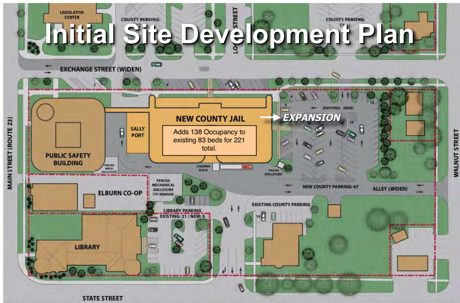
NEW COUNTY JAIL PROPOSED SITE WORK - PHASE 1 TOTAL COUNTY PARKING = 277 +/- TOTAL LIBRARY PARKING = 26
